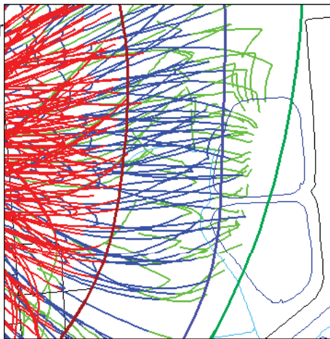
Sensitivity of Particle Traces to Lagoon Recharge Rate Cataraqui Source Protection Region Lansdowne WHPA & Tier 2 WB Study
